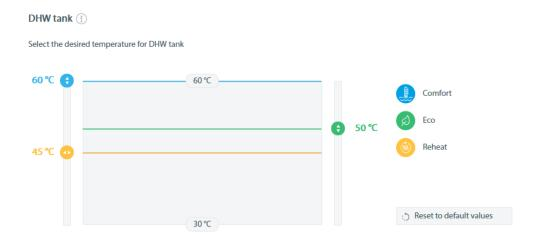
On top of the above the unit is set on a weekly basis to perform the "disinfection function" by raising the temperature in the tank up to 60°C for 1 hour. If an AH-00 fault occurs this typically means the system was unable to complete this "disinfection function" possibly because the hot water was being used during the same period. The system will automatically try to carry out the function another time so the error should pass.
